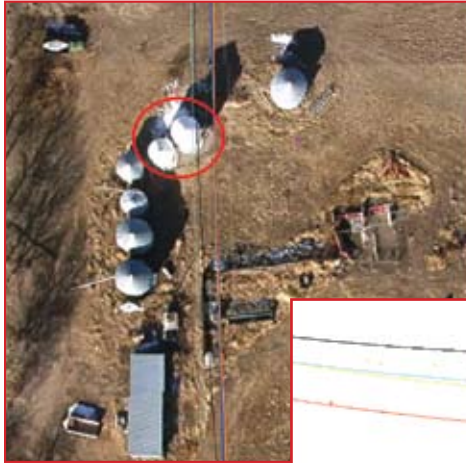
Images of grain silos (storage bins) located on a farm in western Canada with a 138 KV transmission line directly overhead. The profile view, displays the LiDAR points at the time of survey; note the red colored points which are the collected LiDAR wire hits. They are approximately 1.5m above the top of the silo. The solid-colored lines represent the conductor at 100 degrees Celsius, a projected hot temperature that we can predict by using the computer model; note the red phase wire at 100 degrees Celsius combined with a slight side wind would make contact with the Silo. This situation was remedied before any accidents occurred.
