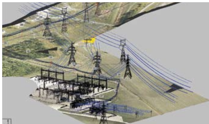
LiDAR data sample, point clouds. The picture at left displays the points once they have been visually classified into specific objects such as tower structures, wires and substation equipment. It has the orthographic imagery laid on top of the digital terrain model, which is a surface model derived from the collected ground points. The picture at right displays the LiDAR points at a low level of classification in which the points are coded based on elevation and object shape. No orthographic imagery is used to aid in the point classification.
