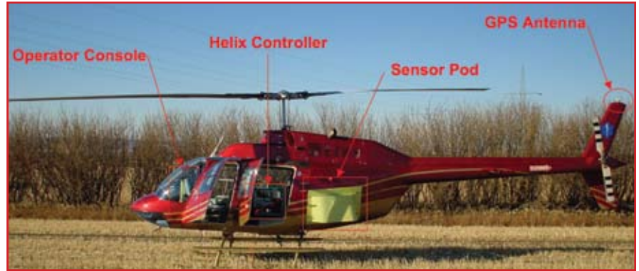
This shows a typical LiDAR installation on a Bell 206B helicopter. The installation can be completed in about six hours, which allows for quick access to project sites.
